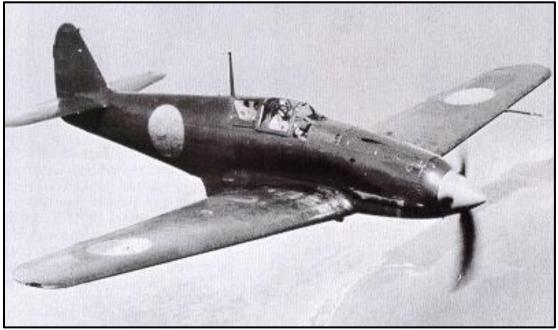
Only liquid cooled in line V produced by Japan. US thought it was a 109. This was a high performing plane that proved Kurt Tank's notions. In the harsh combat conditions of SE Asia and the Pacific, it was a nightmare to keep operational. 18/30 sent from Truk to Rabaul lost in transit. High incidence of non-combat losses. But when it DID work, Allied pilots hated it and recognized it as a high-performance aircraft.
