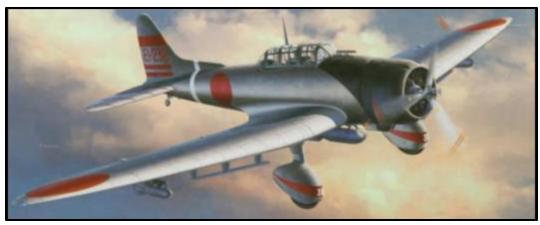
The D3A Val was Japan's primary carrier-based dive bomber and participated in virtually every battle in which the Imperial Japanese Naval Air Force was engaged – beginning with Pearl Harbor. It was an early design, as reflected by the non-retractable landing gear and relatively short range. It was slow by the standards of more recent Japanese and US designs and was no match for US fighters, but despite its limitations it accounted for more US ships sunk than any other Japanese aircraft.
